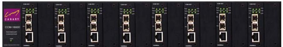
Eight Installed RJ-45-to-Fiber Uni-Directional [One-Way] Converter Cards
